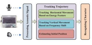
Fig. 7. The workflow of VPad
