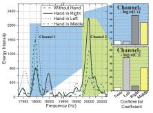
Fig. 2. Illustration of the confidential coefficients of the acoustic signals under different hand positions.
