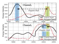
Fig. 6. Doppler frequency shift when the hand movement at the left of the virtual writing tablet.
